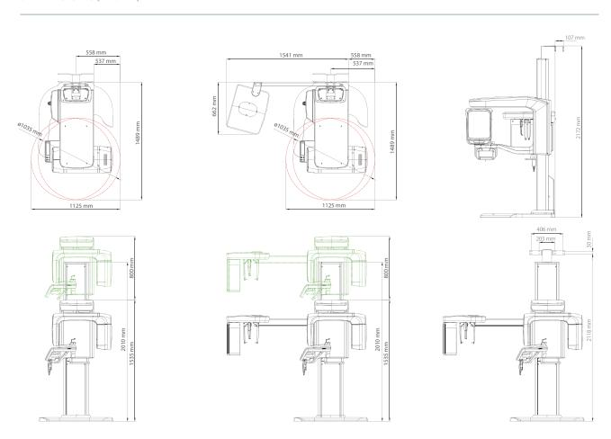
\*An additional 3 inches (76.2 mm) of space is required behind the unit for wall mount bracket installation (mandatory unless there is a base mount installation).
